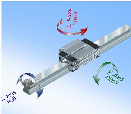
True high-precision performance with linear guides is only possible by limiting unwanted motion in the X, Y and Z axes as the runner block travels along the rail. Rexroth achieves this by optimizing ball recirculation inside the Ball Rail runner block.
