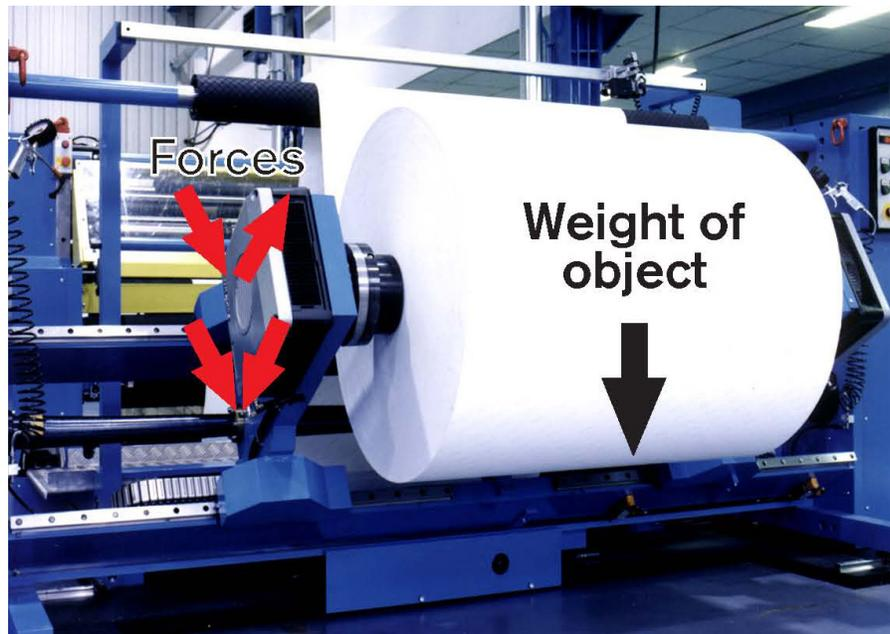
Axial or torsional loading, for example, may require wider or heavier-duty components than simple radial loading.
