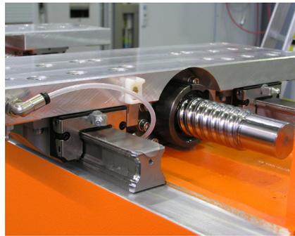
Ball screw and rail combinations like this provide a good balance of travel accuracy and load carrying capability, even with axial or torsional loading.
