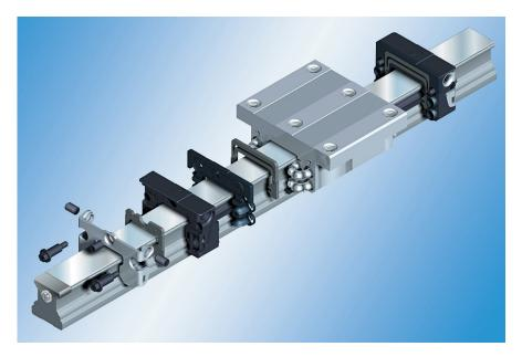
Linear guides house recirculating ball or roller bearings in a runner block mounted on a profiled rail. Some linear guides have multi-part seals to keep lubrication in and contaminants out.
